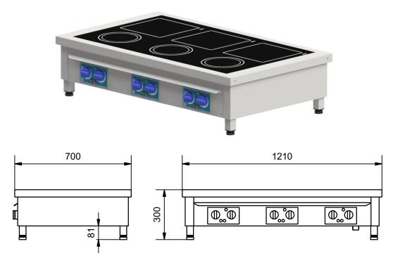
See under the paragraph 'Dimensions for installation' about requirements for space around the appliance.
