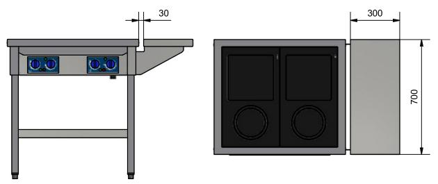
Ranges with two zones and side shelf must be fixed to the floor and cannot be equipped with electric height adjustment.
