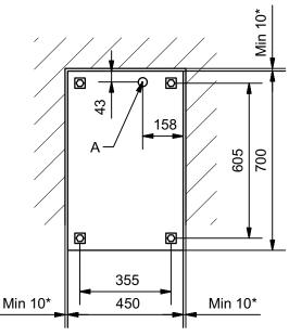
A: Minimum 800mm electrical cable over the floor.
