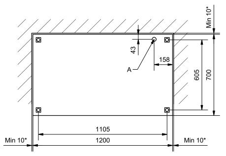
A: Minimum 800mm electrical cable over the floor.
