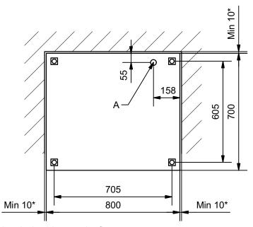
A: Minimum 800mm electrical cable over the floor.
