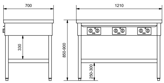
See under the paragraph 'Dimensions for installation' about requirements for space around the appliance
