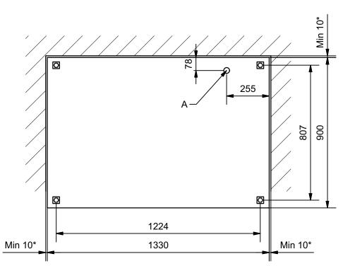
A: Minimum 500mm electrical cable over the floor.
