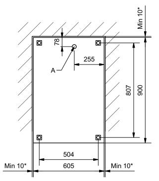
A: Minimum 500mm electrical cable over the floor.
