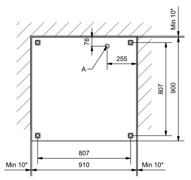
A: Minimum 500mm electrical cable over the floor.
