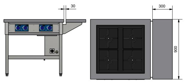
Ranges with two zones and a side shelf must be fixed to the floor.
