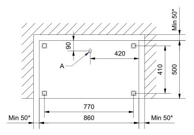
A: Minimum 850mm electrical cable over the floor.
