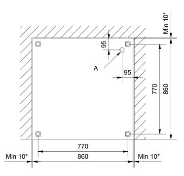
A: Minimum 1200mm electrical cable over the floor.
