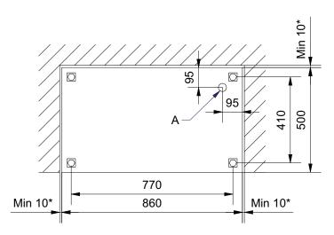
A: Minimum 1200mm electrical cable over the floor.
