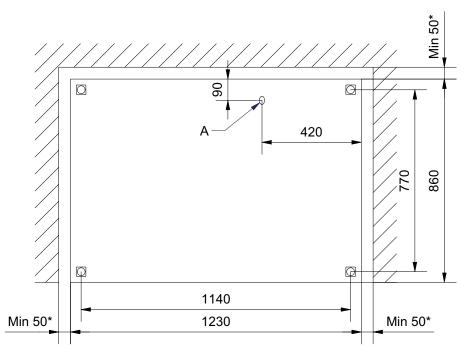
A: Minimum 850mm electrical cable over the floor.
