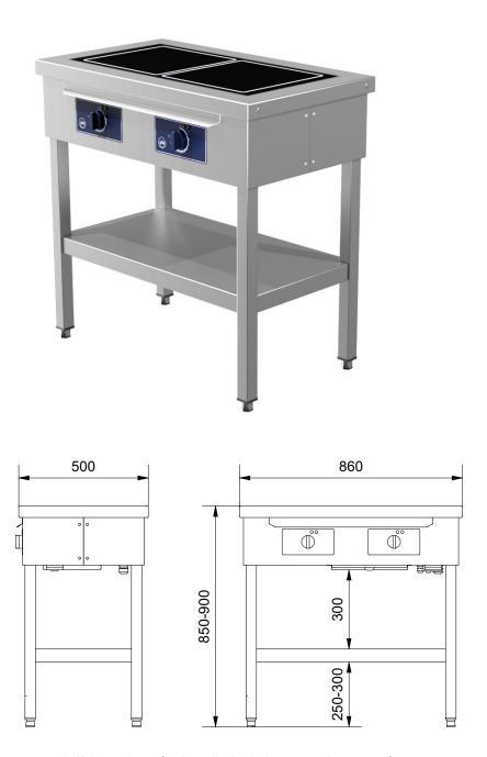
See under the paragraph 'Dimensions for installation' about requirements for space around the appliance.
