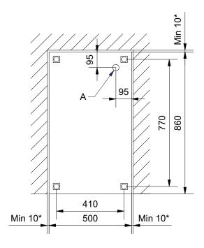
A: Minimum 1200mm electrical cable over the floor.
