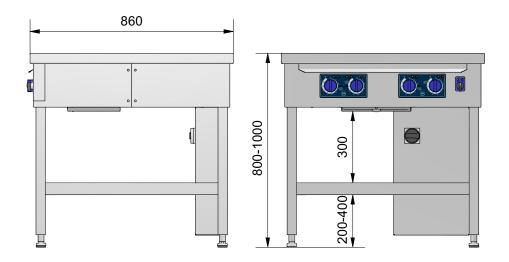
See under the paragraph 'Dimensions for installation' about requirements for space around the appliance.
