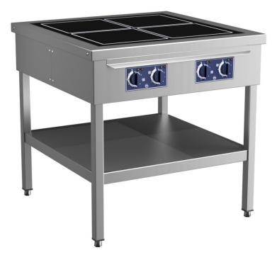
IN 860 is available with square, floating induction zones of 31x31 cm and a power of 5 kW per zone. All sizes can be supplied with a regular stand or with height adjustment (Vari) or as a tabletop model (TT). Ranges with 2 zones can be supplied with control on the long side (SB).
