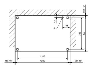
A: Minimum 800mm electrical cable over the floor.
