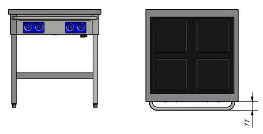
The accessory requires floor mounting and cannot be combined with electric height adjustment.
