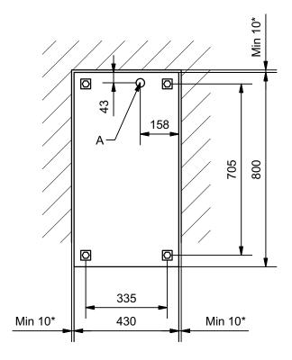
A: Minimum 800mm electrical cable over the floor.
