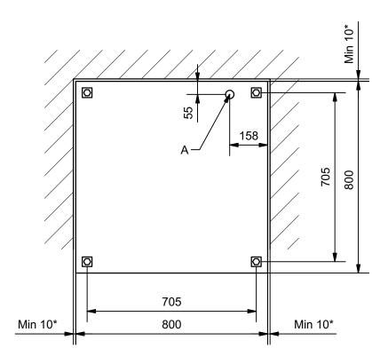
A: Minimum 800mm electrical cable over the floor.
